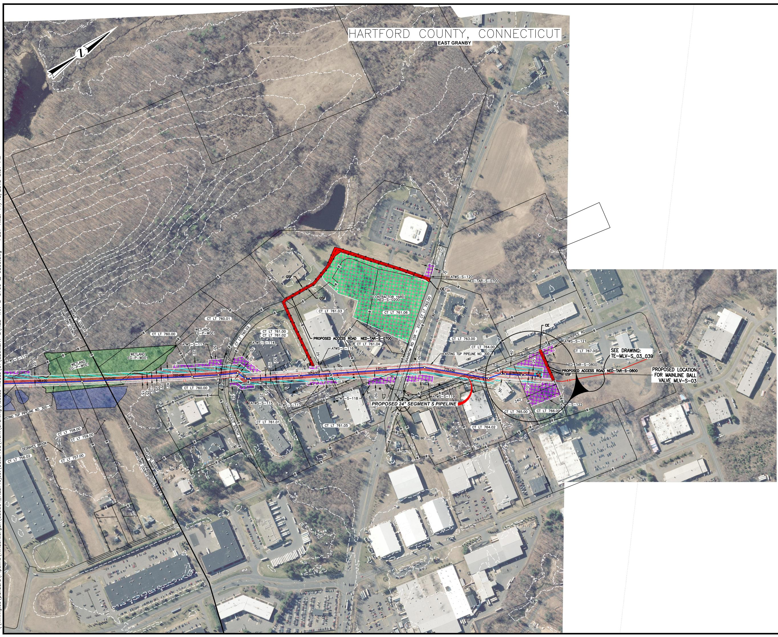
EXISTING PERMANENT EASEMENT PROPOSED PERMANENT EASEMENT TEMPORARY WORKSPACE ADDITIONAL TEMPORARY WORKSPACE (ATWS) POTENTIAL STAGING AREA \_\_\_\_ LIMITS OF DISTURBANCE \_\_\_\_\_ ACCESS ROAD PROPOSED PIPELINE EXISTING TENNESSEE GAS PIPELINE EXISTING FOREIGN PIPELINE OVERHEAD POWER LINE (PA HG3 400.00) LINE LIST NUMBER
